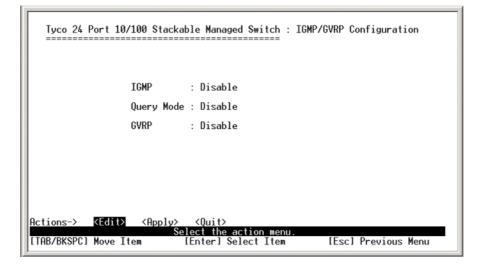
Figure 35. IGMP/GVRP Configuration Screen
